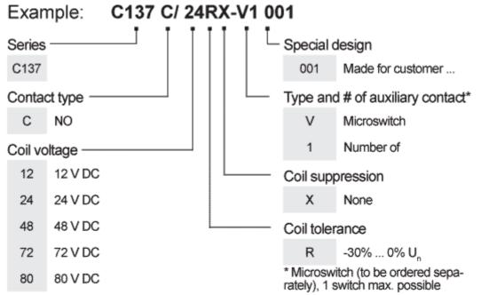
Type C contactors are NO contactors fitted with magnetic blowout. Here the NO contact functions as circuit-breaker within an open contact design.
